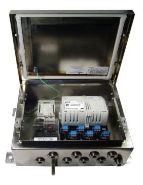
**The key modular components** of the system (Fieldbus Barriers and Surge Protectors) may be 'hot-plugged' by design and without gas-clearance procedures or separate isolating switches. This virtually eliminates the risk associated with hazardous area maintenance activities, speeds module replacement and avoids the need for specialist operator training.
