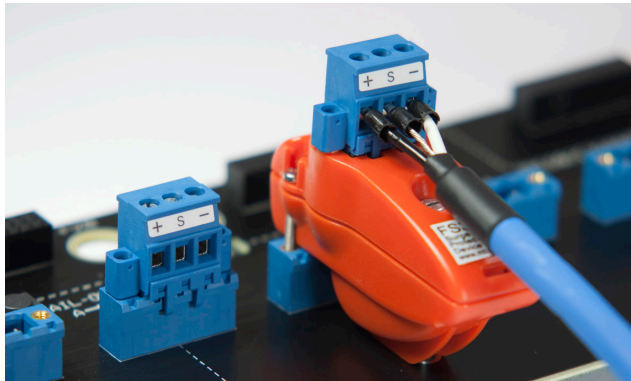
Figure 4.7 - FS32 Spur Surge module on carrier
