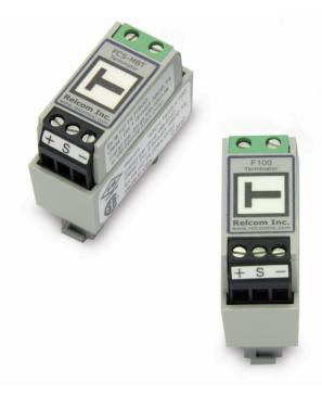
**The fieldbus standards** require that buses must be terminated at both ends to prevent signal reflections. Usually one terminator is provided by the power conditioner in the control room. The MTL range of fieldbus terminators are ideally suited to provide the Terminator that is normally in a junction box in the field (along with a Megablock for interconnecting devices). A large "T" is placed on all terminator labels for easy identification of the Terminator location.
