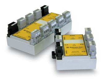
**Short circuit protection** Megablocks are available with built-in SpurGuard<sup>™</sup> short circuit protectors which prevent a short circuit in any of the individual AS-i devices or spur cable runs from bringing the entire network segment down. A red LED near each spur connection indicates that a spur is shorted and is in overcurrent mode.
