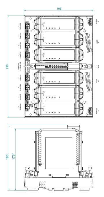
\*This dimension applies if the F809F-Plus diagnostic module is not used.
