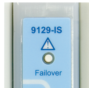
Figure 5.1 SAM failover switch button
