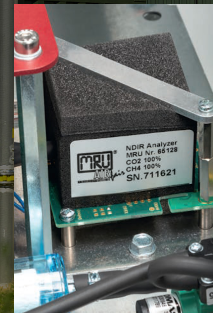
NDIR-bench for CH 4 /CO 2 analysis, for biogas and landfill gas measurements
