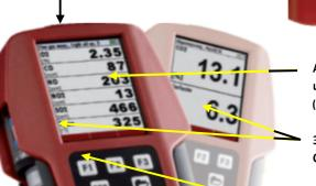
Active CO Sensor protection using 2nd internal pump (not possible with NDIR module)
