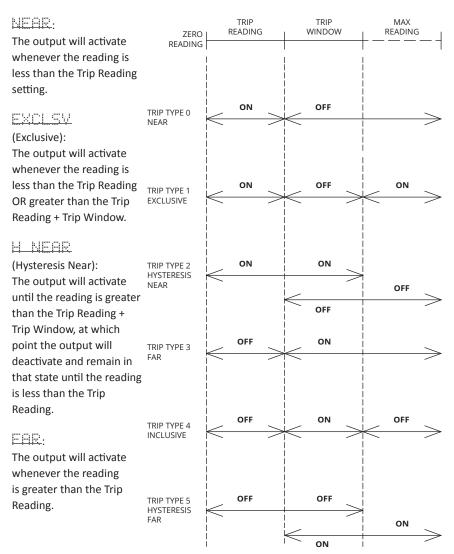
NOTE: for Normally Closed relays, the active state--ON--is Open, and for Normally Open relays, the active state is Closed.
