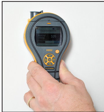
Figure 3: Taking Relative Moisture Readings
