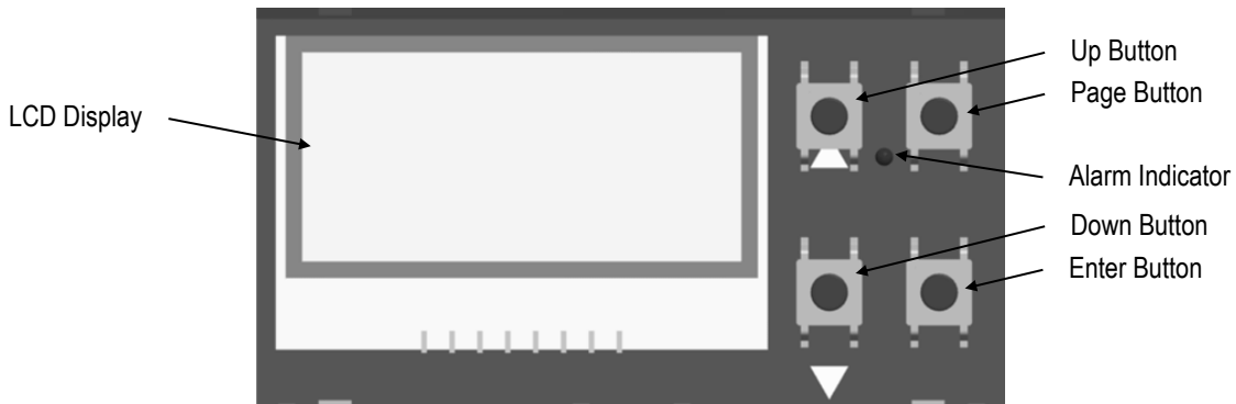
Figure 33: Control Panel for the Comm Box (DIN)
