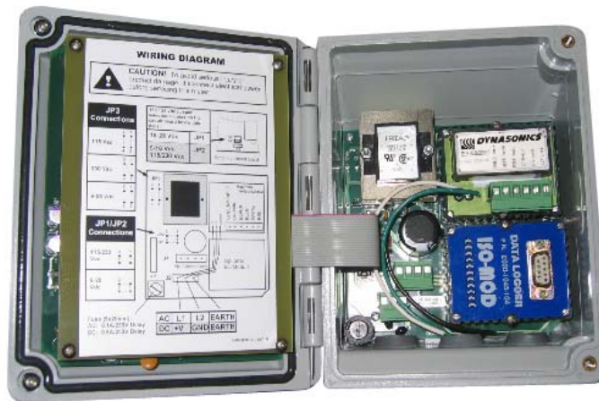
Figure 1.10 Two ISO-MOD I/ O Modules Installed
