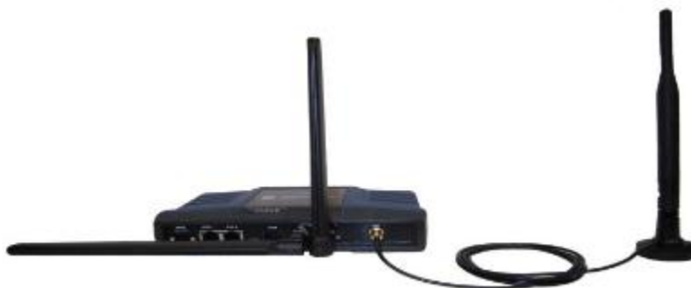
Figure 2-11. Direct Mounting of Cell Antenna; Cabled WiFi Antenna Minimum 8-inch (20.32 cm) separation between cell and WiFi antennas
