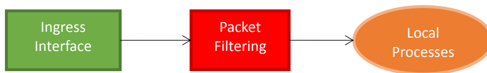
Figure 3-126. Packets Terminated at the Unit
