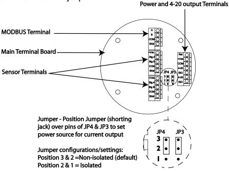
**Warning** Always ensure that JP3 and JP4 jumpers are in the correct position depending on the current output configuration chosen.
