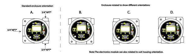
When determining suitable enclosure orientation for specific application, installers should observe all local regulations and quidelines for mounting enclosures.
