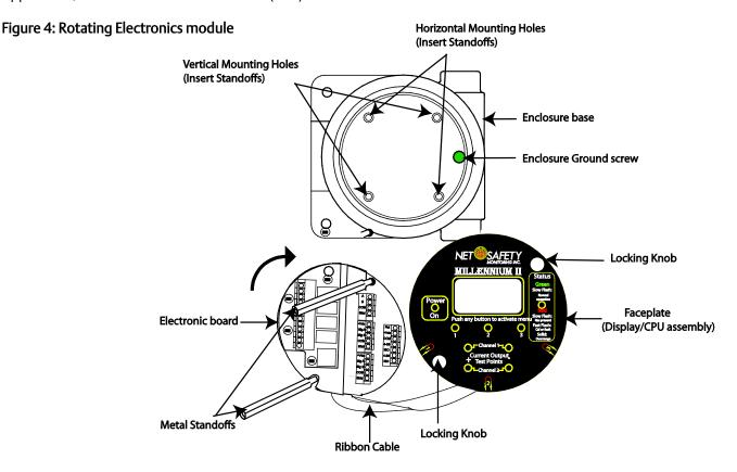
**Note:** To access enclosure grounding screw, remove the electronics module by following steps 1-7 above.
