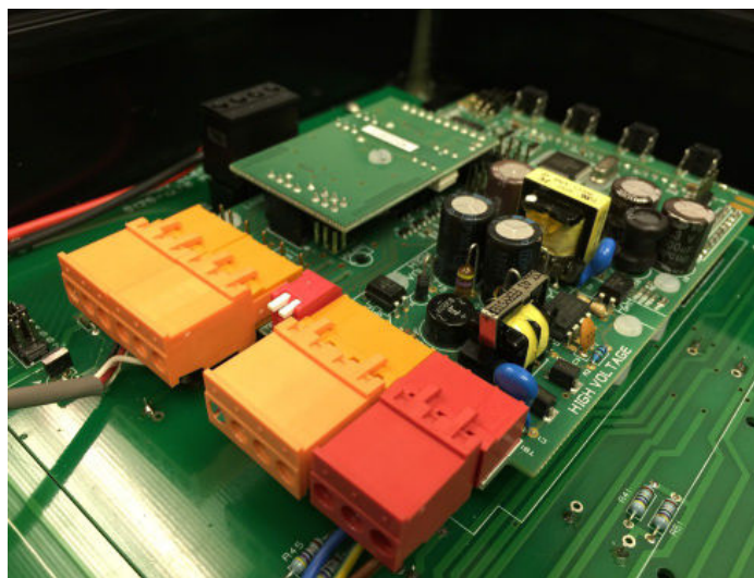
Data connection to MAGNA RS485 input port (upper left)
