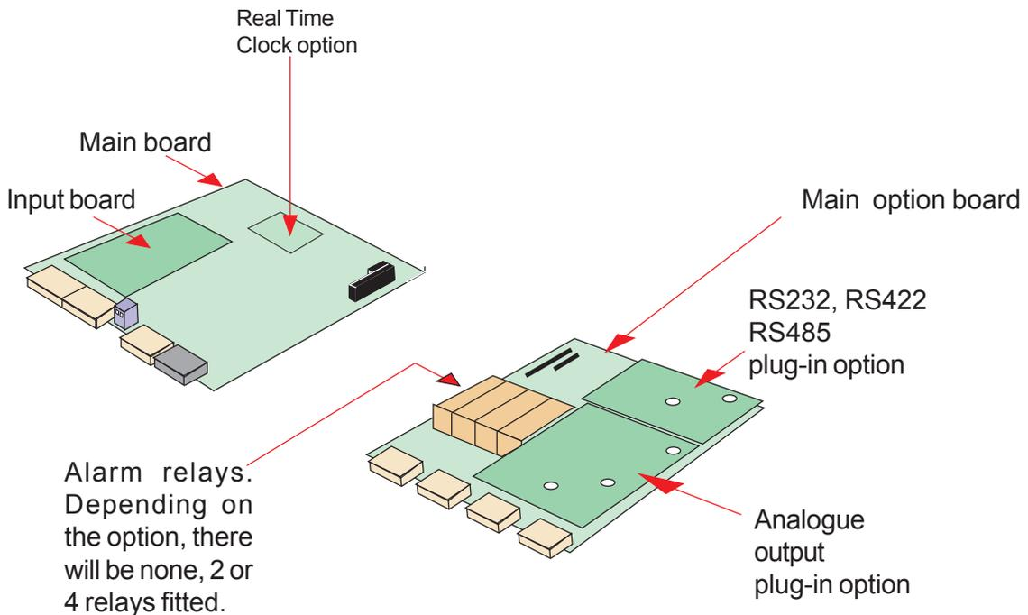
The analog output and RS232 or RS422 plug-in option boards are fixed to the main option board with white plastic pillars. You must apply a firm force when fitting or removing these options.
