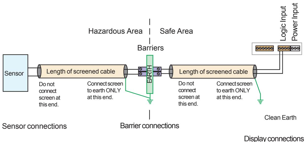
When using multi-core screened cable to connect several displays to several sensors, please be sure to use one twisted pair for each display and sensor.
