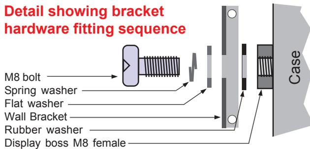
The side holes in the two brackets are 8.5mm dia. to accept M8 bolts.
