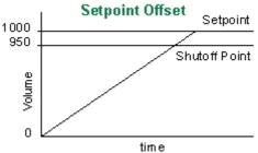
In a repetitive fill operation (as illustrated by example), a setpoint offset of -50 allows a shutoff setpoint to be set for 1000 and actual shutoff to occur at 950 if it is known that 50 units will still flow following shutoff. An offset can also be applied to emptying operations.
