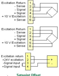
In 4-wire DC or load cell connection, the excitation and sense lines are tied together. The meter can make ratiometric corrections for supply voltage variations, but not compensate for variations in lead resistance. This connection is often used with short cable runs.
