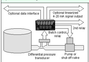
An ideal application for the Extended Laureate VF meter: up- or down- counting batch controller. The dual-relay card is required. One relay is dedicated to batch control, the other relay is available to alarm the rate or total. The signal input can be linear or nonlinear. The display can be toggled between rate and total.
