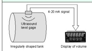
The Extended Laureate VF meter can linearize analog signals for display and alarm using custom curve linearization with multiple nonlinear segments. As illustrated, tank level is measured by an ultrasound detector, which transmits a 4-20 mA signal. This signal is then converted to a highly accurate volume reading. The linearized rate readings can also be totalized.
