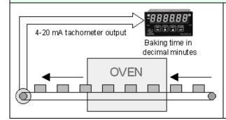
A unique application of the Extended Laureate VF meter: displaying process time based on the 4-20 mA or 0-10 V signal from a rate meter. In the above example, a tachometer transmits the speed of a conveyer belt through an oven. The meter displays baking time in the oven using the relationship time = distance / speed.
