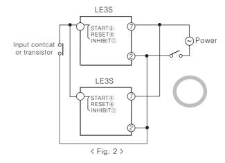
2Please use transformer with primary and secondary isolated power for input.
