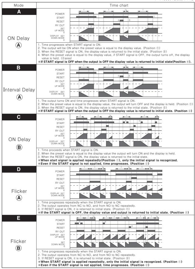
\*Initial state: The output is OFF, the display value is "0". (At Up mode)
