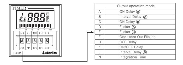
See B−15 and B−16 for the specification information of output operation mode.
