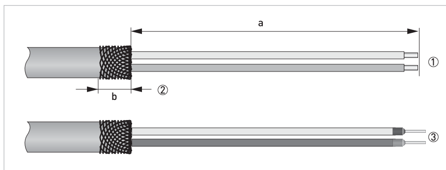
Figure 3-9: Preparation of field current cable C
