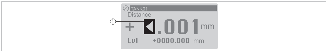
Figure 6-2: Error symbol: the number of digits and decimal places is not sufficient for the measurement data
