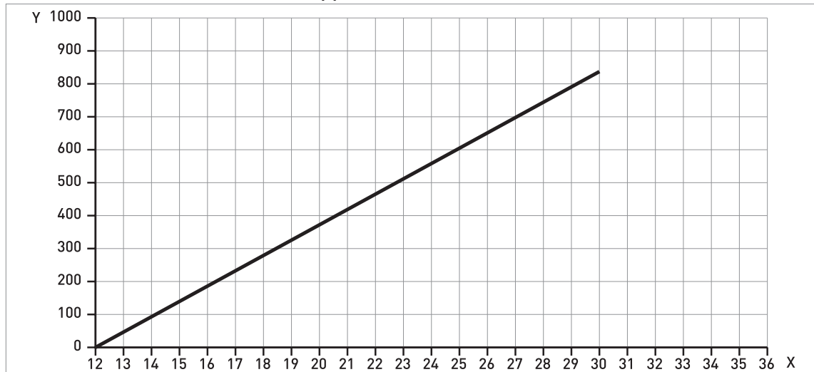
Figure 8-2: Minimum power supply voltage for an output of 21.5 mA at the terminals (Non-Ex and Hazardous Location approval [Ex i / IS])
