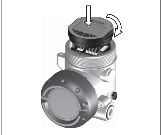
Fig. 21: Installation of the indicating/adjustment module
