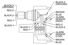
**DUAL ALARM WIRING DIAGRAM**
