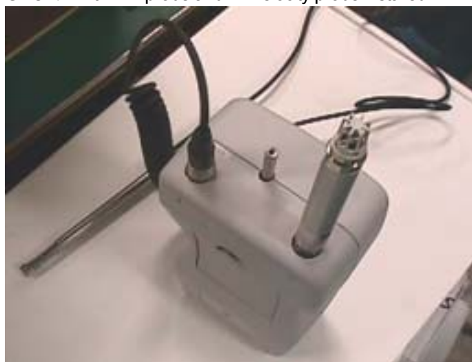
GEO- \alpha with T/H probe and Air velocity probe installed
