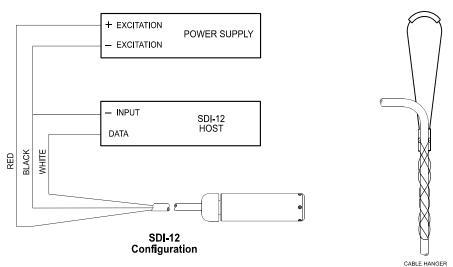
*Note:* This diagram depicts a typical installation. Refer to your power supply and instrumentation manufacturer for the specifics of your application.
