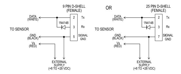
Sensor Connections to 9-Pin and 25-Pin D-Shell RS-232 Serial Port
