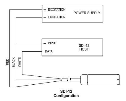
Note: This diagram depicts a typical installation. Refer to your power supply and instrumentation manufacturer for the specifics of your application.
