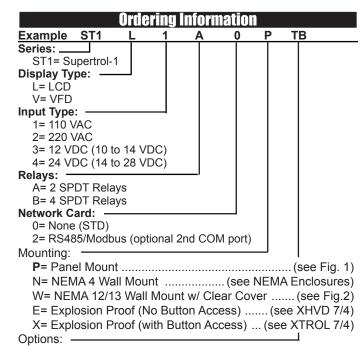
TB= RS485 Terminal Block for Panel Mount Enclosure
