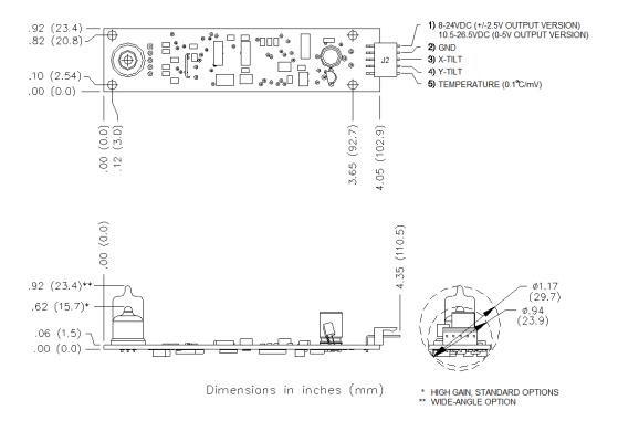
A901, Slimline Biaxial Clinometer (Horizintal Configuration)
