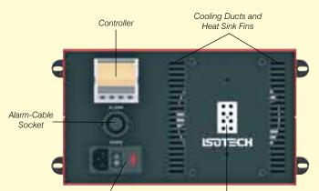
Switched Mains Cable Socket & Fuse-Holder Metal Block with Pockets for Thermocouple Junctions
