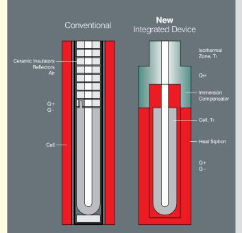
A fixed point cell is not long enough to eliminate heat conductance along the thermometer calibrated in it. Currently, using long furnaces, heat shunts and reflective baffles an attempt is made to reduce these losses.
