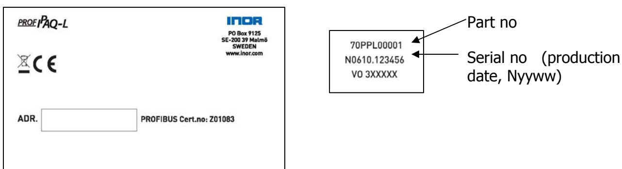
Figure 4 Label 1 and 2 on enclosure of the transmitter ProfIPAQ-HXDxy 70PPHXDxy1 (e.g. 70PPHXD111)
