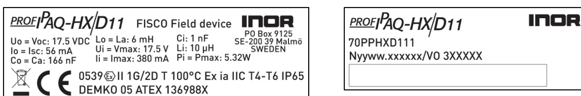
Figure 4 Label 1 and 2 on enclosure of the transmitter ProfIPAQ-HXDxy 70PPHXDxy1 (e.g. 70PPHXD111)
