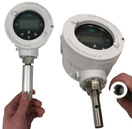
Figure 5: HygroPro XP installation step 1 – removing desiccant cap
