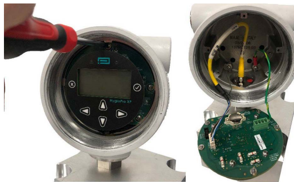
Figure 8: HygroPro XP installation step 4 - unfasten the HMI
