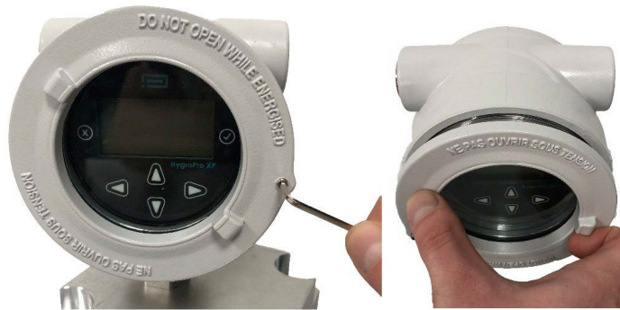
Figure 7: HygroPro XP installation step 3 - loosen the set screw and unscrew the enclosure lid
