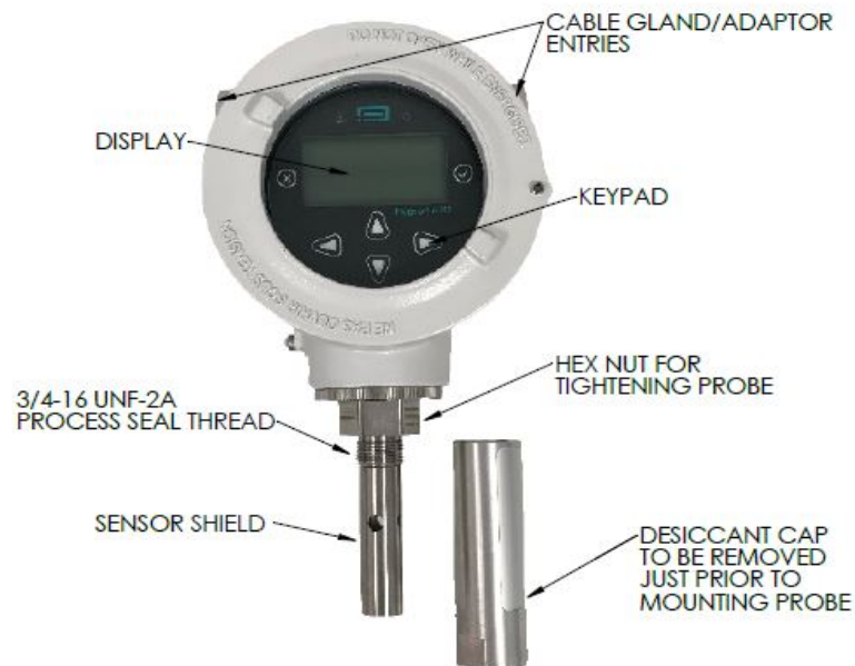
Figure 4: Key HygroPro XP parts relevant to installation
