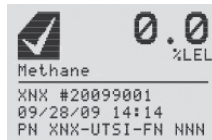
Figure 40. General Status screen with unit information
