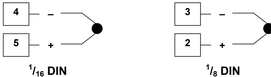
Figure 15. Thermocouple Input Connections
