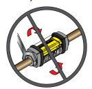
**Never** use wrench to rotate meter body when viewing flow scale
