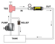
Figure 6: Pump test
