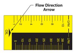
Figure 1: Flow direction arrow
