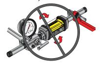
**Never** use wrench to rotate meter body when viewing flow scale
