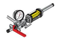
Place wrench on valve body **on the same side** plumbing is being tightened
