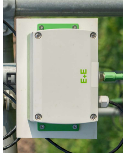
HTS801 unit (without display) after several years of outdoor testing: showing equally positive durability and performance results as the EE310
