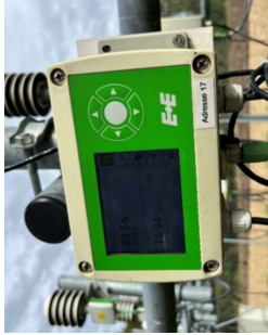
EE310 unit after several years of outdoor operation: minimal weathering and fully functioning display, which is typically the first component to show wear.
