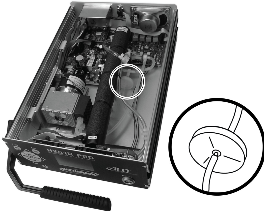
Figure 2-9. NDIR Optical Sensor
