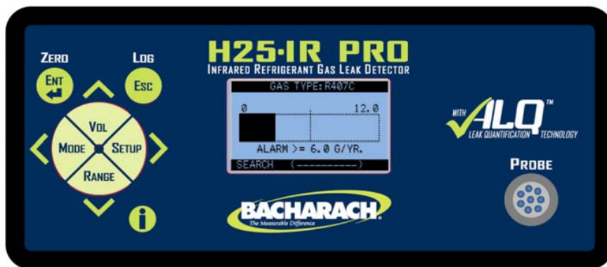
Figure 3-4. Front Panel Components with Sample Display
