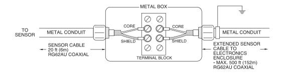
Note: Optional Watertight steel NEMA4 Junction Boxes with terminal strips (Option JB) are also available from Greyline Instruments.
