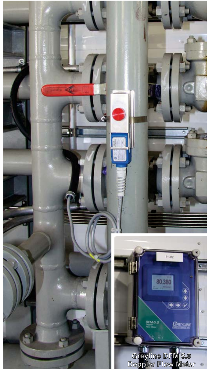
Clamp-on Ultrasonic Transducers Monitoring Crude Oil Flow in 3" Steel Pipe
