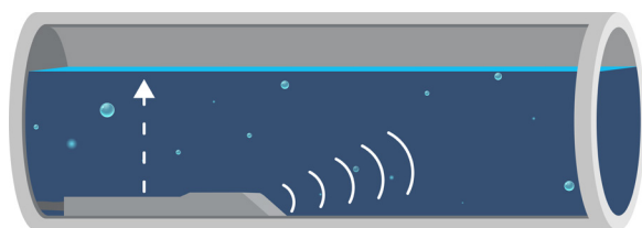
Submerged ultrasonic sensor measures level and velocity
