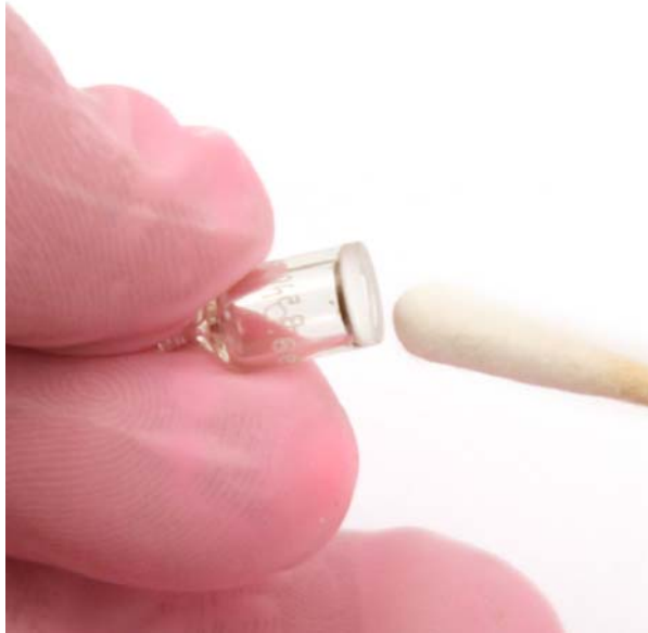
Figure 27: Polishing the Electrode Lamp Window
