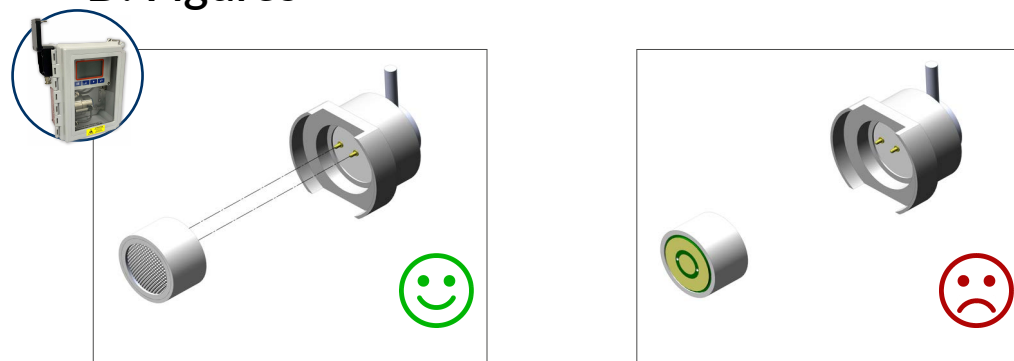
Figure 1 - GPR-1500: Aligning your sensor
