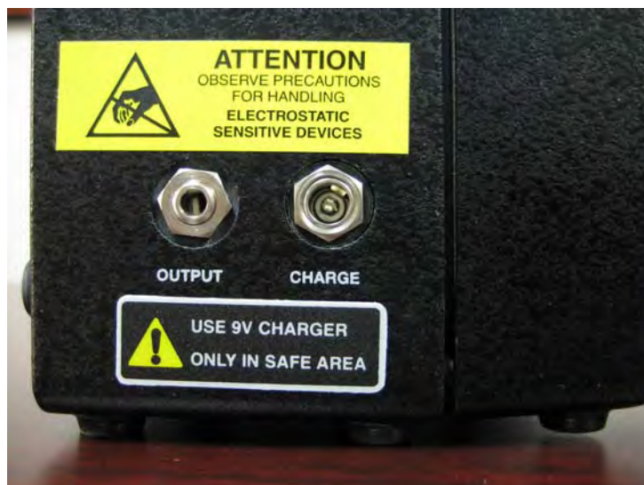
Side of analyzer: signal output and battery charging connectors
