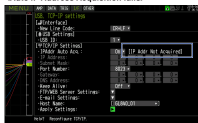
<Auto IP Address Acquisition fails>
