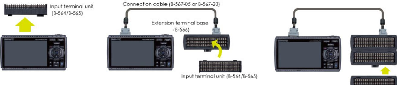
(1)The terminal units is removed from the main body of the GL840.
