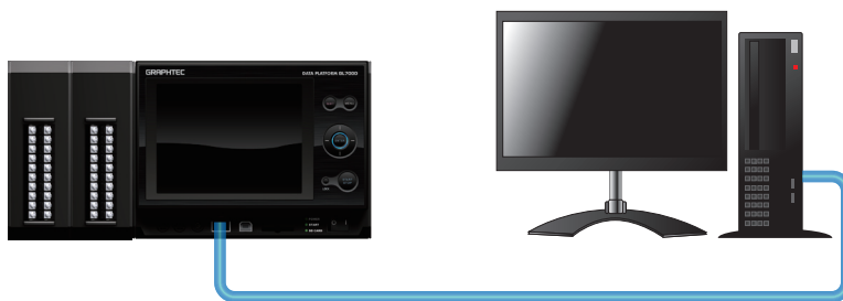
LAN cable (cross over)
