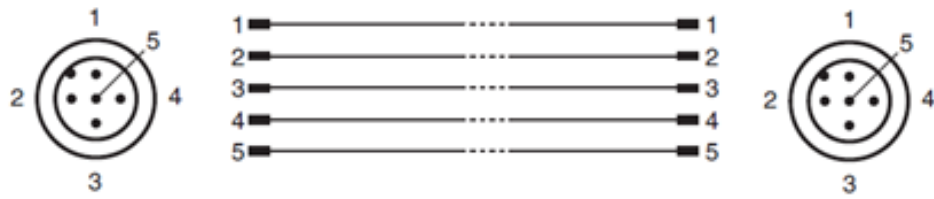
Figure 113: Cable 1 Pin Assignments
