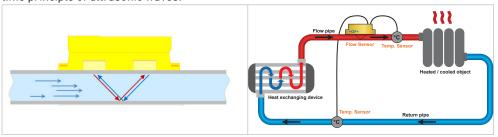
The type U1000 V2  $\,$  functions, as do all current ultrasonic flowmeters, according to the path-time principle of ultrasonic waves.
