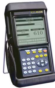
TransPort® PT878 Portable flowmeter
